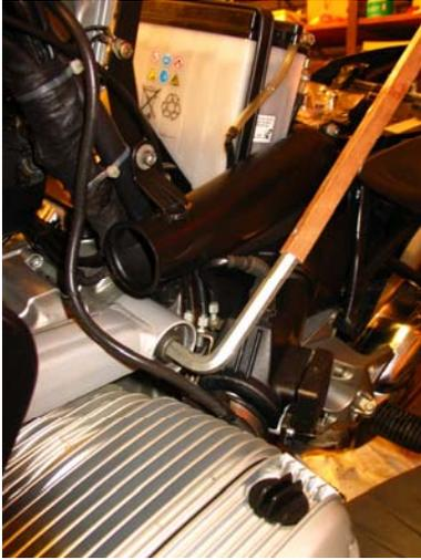
Loosen the left cover with an Allen key
