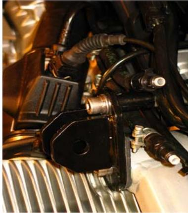
Now place the 33mm tube between the bracket and the high M10 nut. Take the M10x60 Allen bolt, place a spring spacer and spacer over the bolt and screw this into the high M10 nut, fasten with 40Nm. Now fasten the M12 Allen bolt with 73nm.
