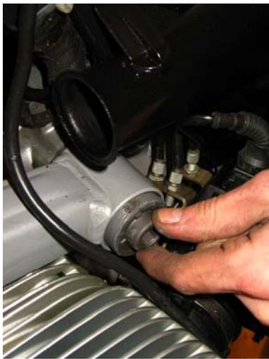
Replace the left cover and tighten with 42Nm.
