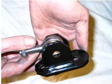
First make sure the 14mm ball joint fits well in the bracket. If not remove sharp edges with a file, when the bracket is to tight grind of the ball of the ball joint until it fits. **You must not bent the bracket!** Of course you will use the grinded ball joint later on this side of the bracket when you are in chapter D.
