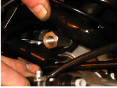
Replace this with the high M10 nut, tighten with 40 Nm.
