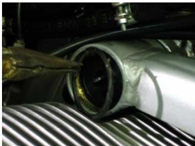
Remove the circlip on the right side....
