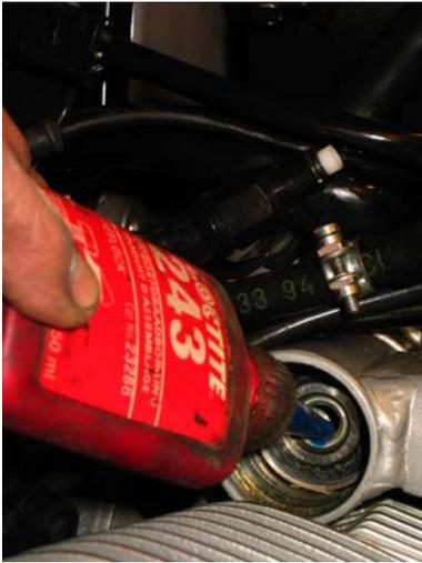
Apply loctite to the thread of the axle from the telelever
