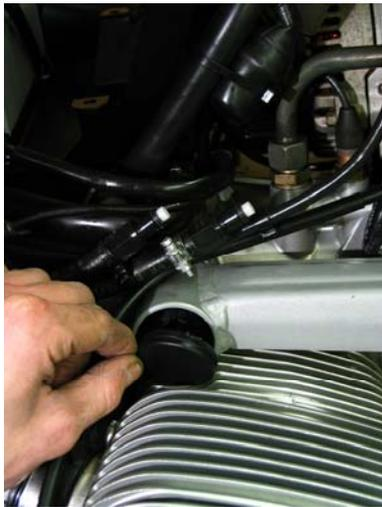
Remove the plastic caps on both sides of the telelever.
