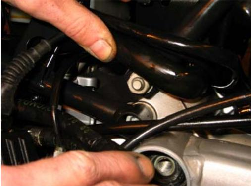
And remove the nut on the right side which connects the front(upper) frame to the engine...
