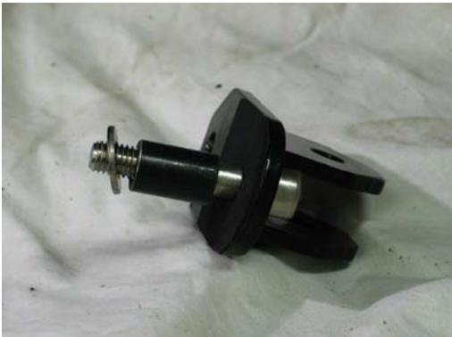
Insert the M12x55 Allen bolt through the centre hole of the bracket. Place the 27mm tube followed by an M12 spacer over the bolt. Place this for the telelever turning point and fasten the M12x55 bolt in the axle of the telelever. **Do not completely tighten and make sure the spacer is mounted correctly!**
